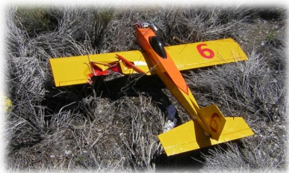
Tony's airplane after the collision. Rick's prop chewed up the left wing—the damage could have been worse.
