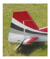
Fly some flat figure-8s in the sky and watch to see how the plane reacts. If you're turning to the left and the plane climbs, you need to add left rudder trim. If the plane dives, add right rudder trim. If you are turning to the right, and plane climbs, add right rudder trim; likewise if it dives, add left rudder trim. Fly flat figure8s until your plane performs smooth turns during right and left banking.
