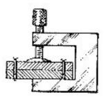
Before laminating plywood for firewalls, lightly clamp and drall two holes a shade smaller than the two nails. Gloe the pieces together, tap in the nails to prevent the parts from skidding then clamp firmly. Once the glue is set, remove the nails and fill the holes. Ruy MrGuckin, Fairport, New York.
