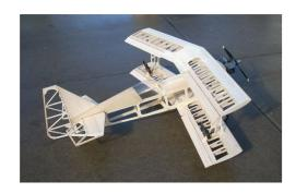
With a Super Tiger .90 2 stroke or a .91 four stroke and Futaba gear.
