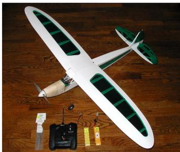
This is a Radio Controlled, Electric Powered, Ready-to-Fly Rascal. Needs: Charger to charge the 8 cell (7.2v) NiCad battery packs
